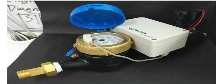
Smart Water Meter
